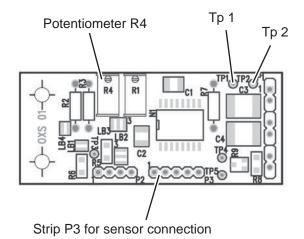
Fig. 7-15: OXS Board, Top View
